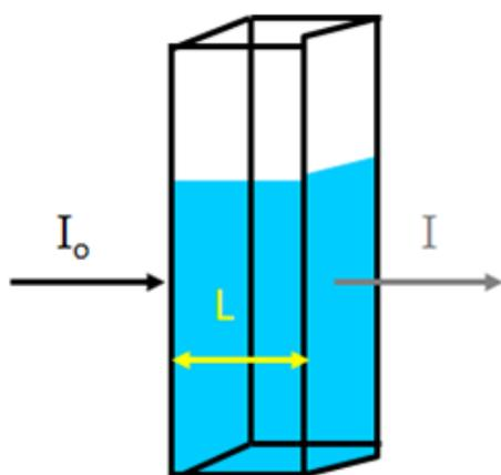
Figure 1 Basis of a uv vis measurement
