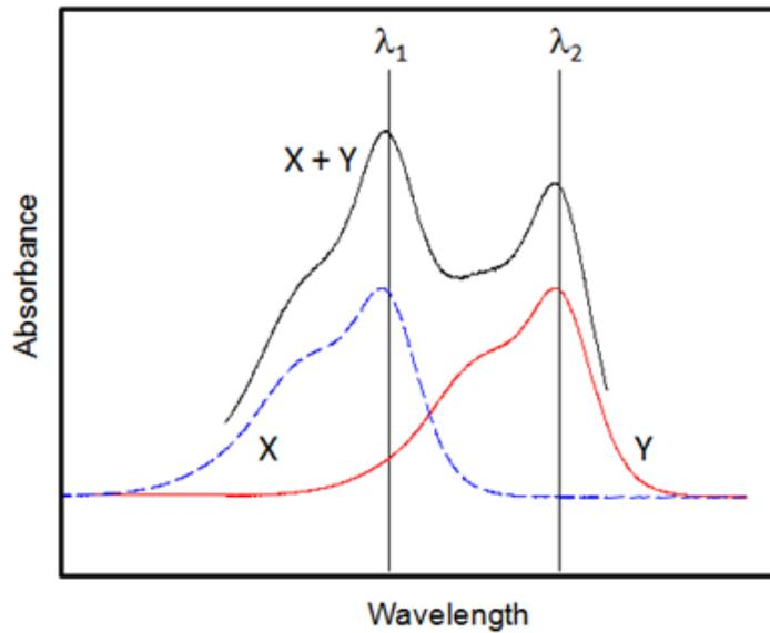
Figure 4: The spectrum produced by a mixture of components X and Y. Analyses wavelengths for the mixture,  $\lambda_1$  and  $\lambda_2$  are also shown.
